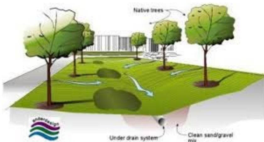
Figure 4.4 - A typical swale (Sudswales.com)
